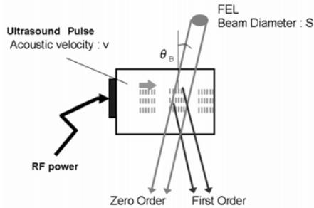
Figure 2: Principles of an AOM.
