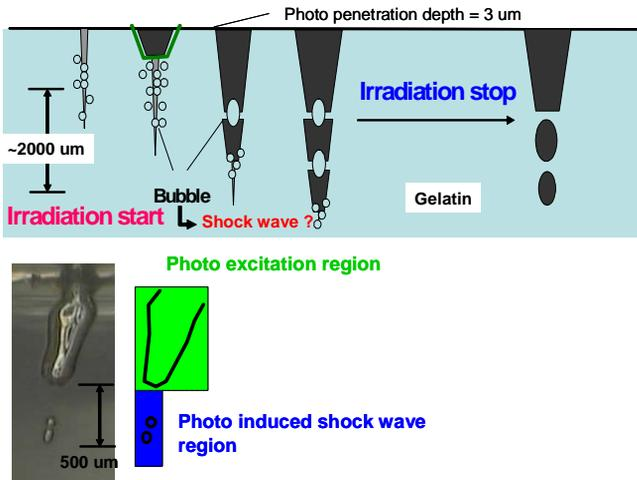
Figure 6: The process of gelatin cut.
