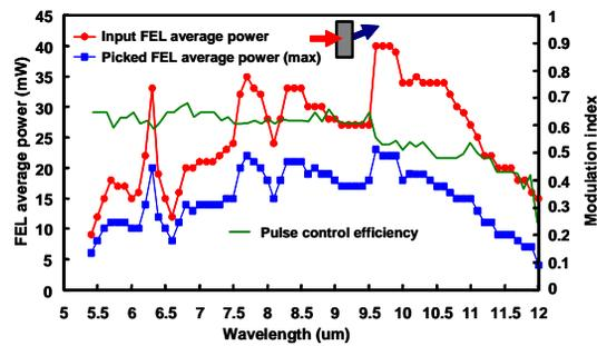
Figure 4: Wavelength-dependence of pulse control system.
