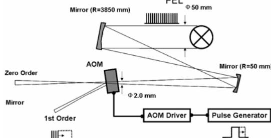
Figure 3: Experimental setup for pulse control.
