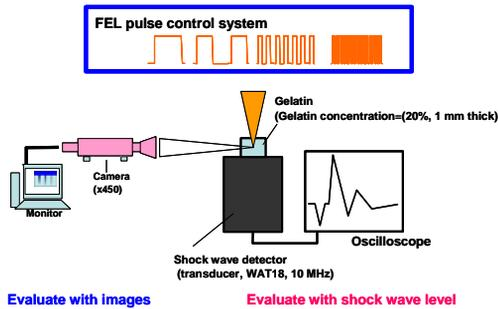
Figure 7: Experiment setup for proof experiment of pulse control effect.
