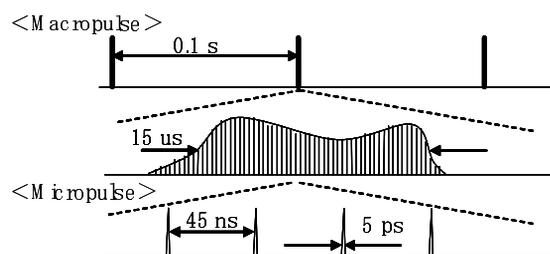
Figure 1: Pulse structure of FEL.
