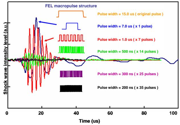
Figure 8: A difference of a level of shock wave by a difference of pulse structure.
