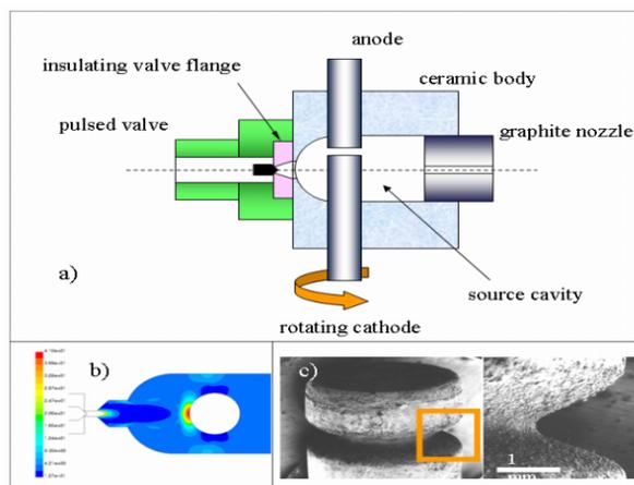
Fig. 2: a) schematic diagram of the PMCS source; b) pressure contour plot of He jet inside the PMCS cavity (see ref [11]); c) scanning electron microscope micrographs of the cathode region eroded by the plasma. The cathode is continuously rotated in order to prevent the formation of holes. A very smooth and precise trace formed by plasma erosion is clearly distinguishable.
