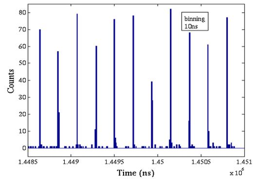
Figure 5: Expanded view of the microtemporal structure of photon count peak under FEL giant pulse in the Q-switch mode.
