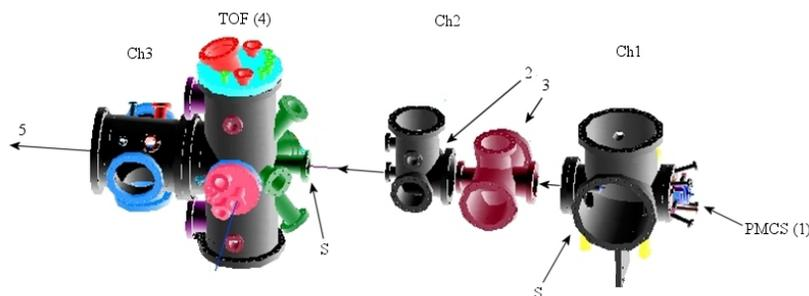
Fig. 1: Main elements of CESyRA apparatus: (Ch1) expansion chamber, (Ch2) deposition and gas exposure chamber, (Ch3) TOF, (1) PMCS, (2) manipulator, (3) gas line, (4) TOF, (5) to dumping chamber and quartz microbalance.
