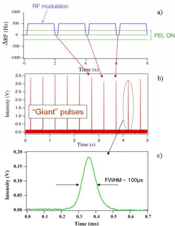
Fig. 3. Q-switching of the SRFEL: a) the RF modulation can be triggered by the opening of the He valve of the clusters source, b) development of a sequence of giant pulses, c) detail of a giant pulse: typical duration is 100  $\mu$ s.
