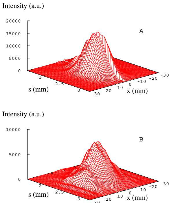
Figure 2: Radiation intensity just after reflection on the upstream mirror (A) and just before the undulator's entrance (B) as a function of the horizontal cross-section (at  $y=0$ ) and the position within the optical micro pulse  $s$  after 75 round trips and for  $\Delta L=1.5\lambda$ .
