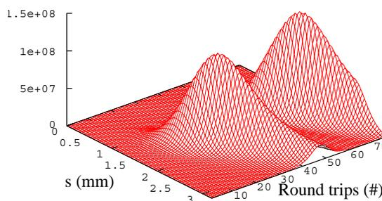
Figure 3: Micro pulse optical power as a function of both the position  $s$  within the pulse and the round trip number for a detuning  $\Delta L=-1.5\lambda$ .
