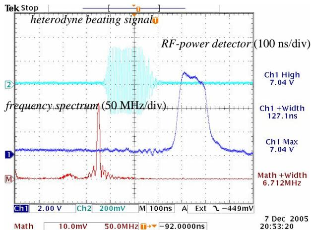
Figure 2: Typical oscilloscope traces of the RF-pulse generated by 30 GHz JINR-IAP FEM.
