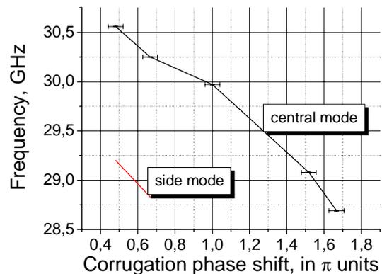
Figure 3: Measured dependence of the FEM oscillation frequency on the value of the phase shift of corrugation between the Bragg structures.
