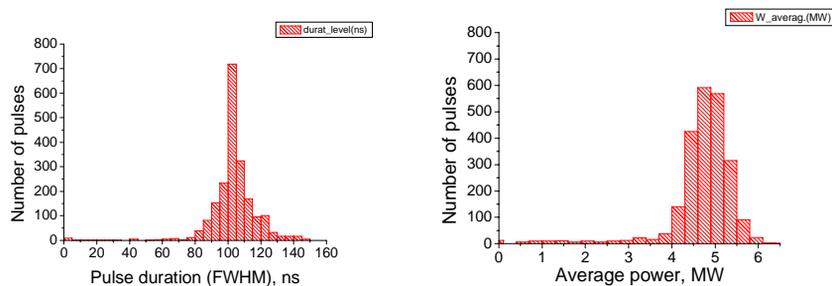
Figure 5: Statistic distributions of pulse duration and RF-power after the test cavity in the series of  $10^4$  pulses.
