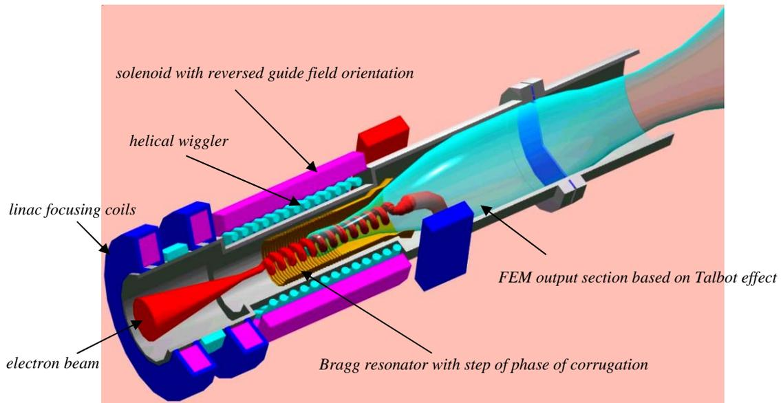
Figure 1: Schematic diagram of the JINR-IAP FEM.
