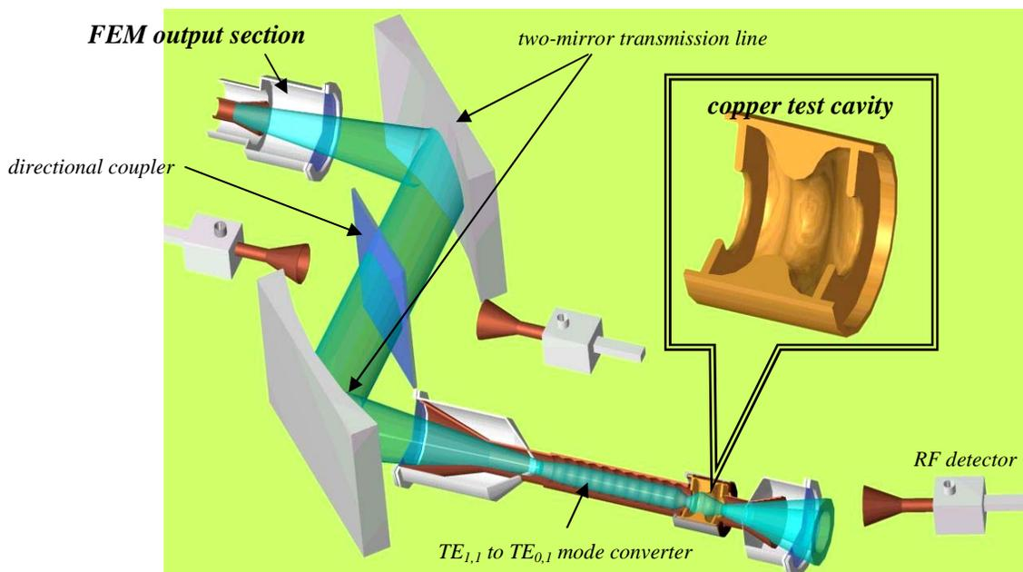
Figure 4: Schematic diagram of the test facility for studying surface heating effects based on JINR-IAP FEM.
