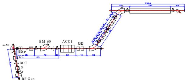
Fig.1: the schematic of the FIR-FEL facility.
