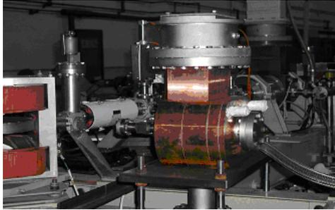
Fig.4: the thermionic cathode injector.
