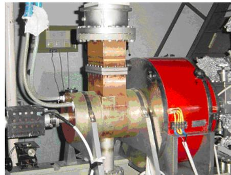
Fig.7: the 4+1/2cell photo-cathode injector.
