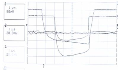
Fig.12: the beam current at the different position on the beam line, measured with BCT.
