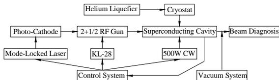
Fig.11: the schematic of the SRF test facility.
