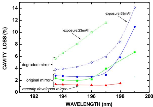
Figure 2: Wavelength dependence of the cavity loss of  $\text{Al}_2\text{O}_3/\text{SiO}_2$  multilayer mirrors. The losses of mirrors manufactured in the previous work are shown by squares and circles, while the loss in the present work is represented by triangles.
