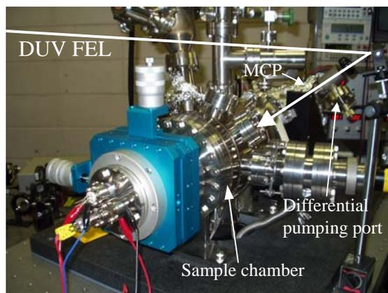
Figure 5: Photograph of the FEL-PEEM system.
