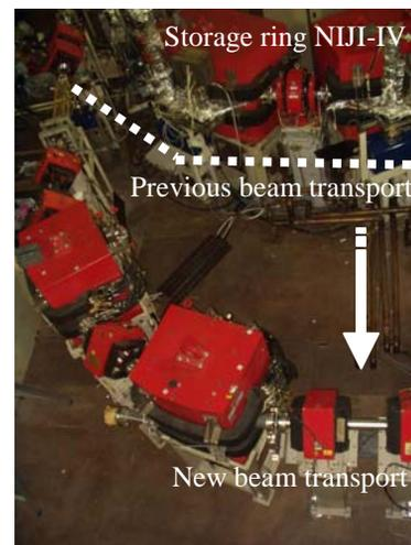
Figure 4: Photograph of a part of new beam transport system. The place where previous beam transport located is indicated by dashed line.
