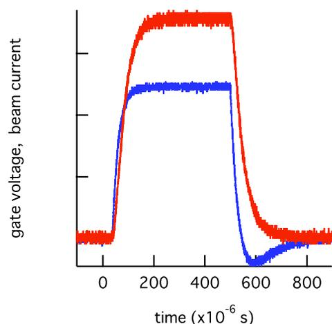
Figure 6: Time trace of the gate voltage (red) and the beam current (blue). Peak voltage is 50 V and peak current is 81  $\mu\text{A}$ .
