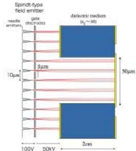
Figure 1: Schematic view of compact CFEL.
