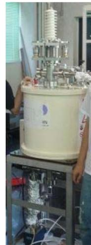
Figure 5: Picture of the CFEL test bench. The high voltage feedthrough, the 2-axis manipulator for resonator alignment and cryostat of the super conducting coil can be seen. The height and footprint of the device are 1.9 m (including a 0.7 m-height pedestal) and  $0.7 \times 0.7 \text{ m}^2$ , respectively.
