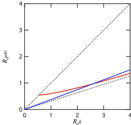
Figure 2: Dispersion relations of the evanescent wave for  $TM_{01}$  mode. The relative dielectric constant of the medium is 10.(red) Both axes are multiplied by the channel radius ( $R_d=25 \mu\text{m}$ ) for the normalization. The blue solid line shows the dispersion of 40 keV beam mode. Upper and lower dashed lines denote the dispersion of the light in vacuum and the light in the dielectric medium, respectively.
