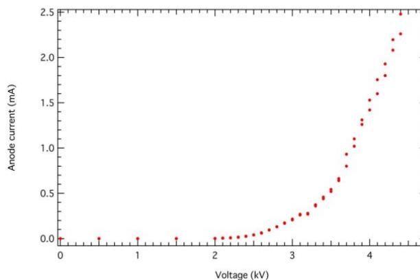
Figure 8: V-I curve for carbon nanotube cathode. D.C. voltage up to 4.4 kV was applied to the collector electrode.
