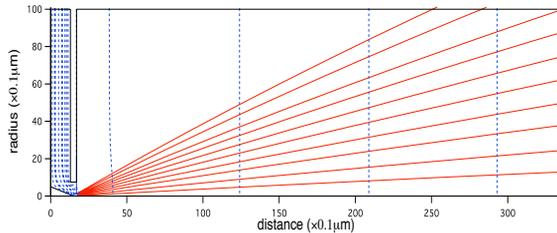
Figure 3: Calculated trajectories of electrons emitted by Spindt cathode. Red lines show the electron trajectories and Blue lines represent the equipotential lines. E-gun code was used for the calculation.
