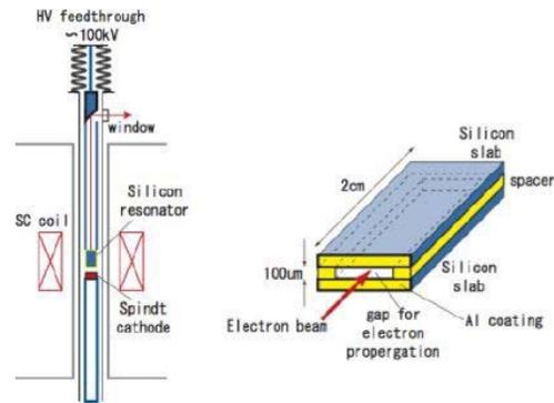
Figure 4: Schematic view of the CFEL test bench and the resonator. The left and right figures show the schematic view of the whole system and the detailed view of the resonator, respectively.
