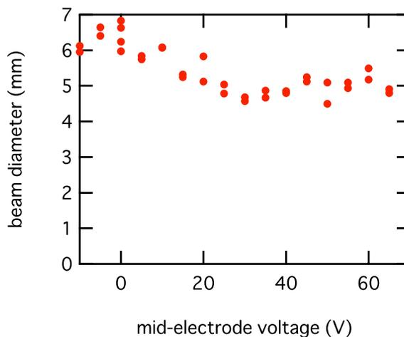
Figure 7: Beam diameter as a function of the mid-electrode voltage. During experiment, the collector voltage was held at 10 kV and pulsed 65 V voltage was applied to the gate electrode of Spindt cathode.
