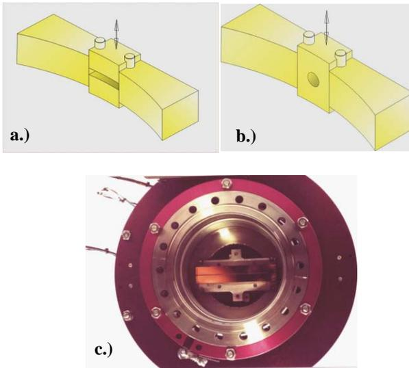
Figure 2 a-c: The lateral dimension of the outcoupler mirrors shown in a.) , b.) amounts to  $\sim 14$  cm. The radius of curvature is  $\sim 3.5$  m. The outcoupler mirror shown in c.) is constructed for an FIR FEL operating at  $\sim 230$ - $650$   $\mu\text{m}$ .
