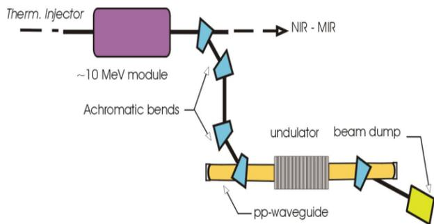
Figure 1: Layout of the FIR-FEL beamline option.
