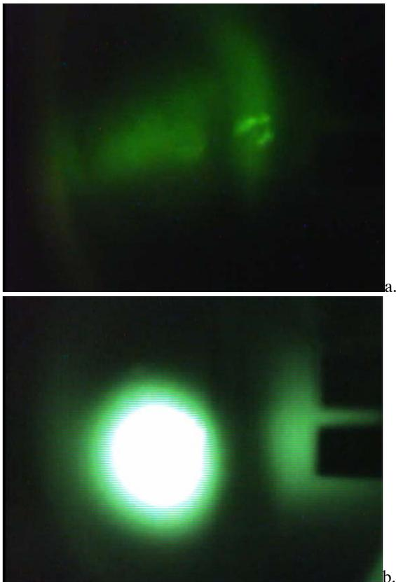
Figure 4. (a) coherent harmonics emitted during fundamental lasing on the output coupler of the laser. (b) Harmonic lasing at 0.53 microns obtained by lengthening the optical cavity by a fraction of a micron.
