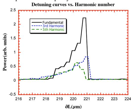
Figure 1. Power vs. cavity length for lasing at the fundamental, third, and fifth harmonic, with fundamental wavelength  $\sim 1.04 \mu\text{m}$ .
