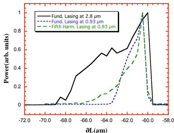
Figure 3. Detuning curves for three different configurations using the 2.8 micron mirrors.
