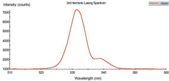
Figure 5. Lasing spectrum using an Ocean Optics visible spectrometer array. This is a single macropulse shot.
