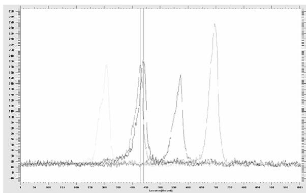
Figure 3. Streak camera images for five different beam energies. The yellow and green curves provide a calibration ratio, beam energy to pixel location. The pink and blue curves demonstrate the high degree of energy resolution of the system. The red curve is the nominal 115 MeV setpoint energy.
