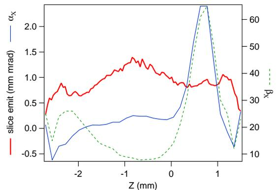
Figure 9: Slice analysis of the emittance,  $\alpha_X$  and  $\beta_X$  parameters for the double peaks solution.
