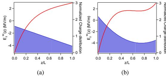
Figure 2: Longitudinal space charge field on axis of a linear (a) and parabolic (b) ramping charged bunch just extracted from the cathode having different radius;  $Q=1\text{nC}$ ,  $L=3\text{mm}$ . Cathode plate is in  $z=0$ .
