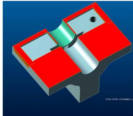
Figure 6: Preliminary technical drawing of the cavity BPM [4].
