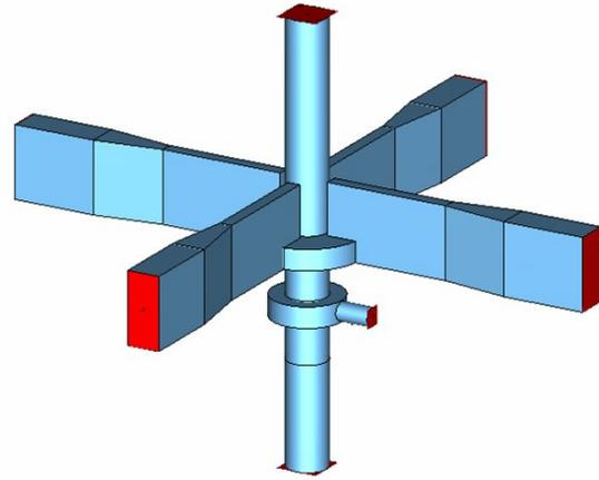
Figure 4: C-band cavity BPM with its four coupling waveguides and reference cavity.
