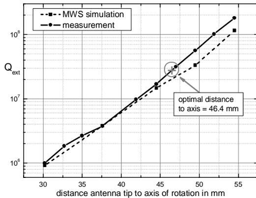
Fig. 3: external quality factor vs. antenna length.
