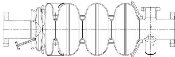
Fig. 1: cross section of the cavity design.
