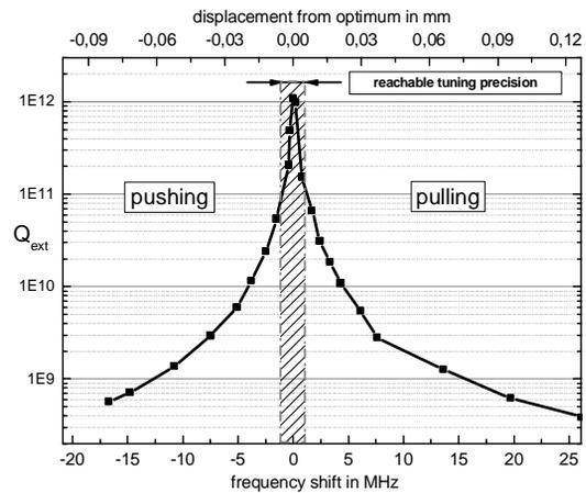
Fig. 4: external quality factor vs. detuning from best  $\pi$ -mode suppression.
