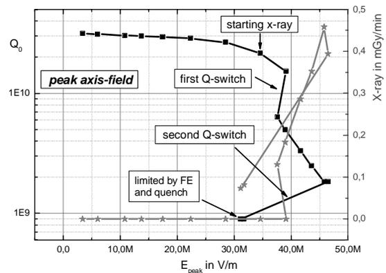
Fig. 8:  $Q_0$  vs. peak axis field  $E_{peak}$  @ 1.8K.
