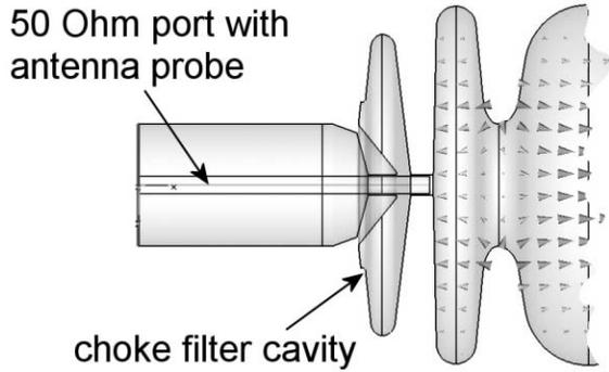
Fig. 5: assembly to measure  $\pi$ -mode suppression.
