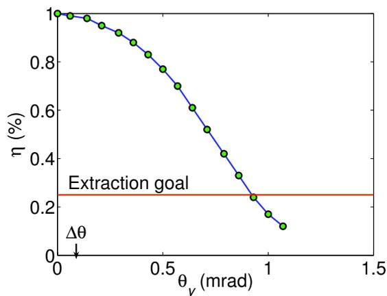
Figure 8: Extraction  $\eta$  vs. electron beam tilt  $\theta_y$  for the proposed BNL FEL. The extraction goal is obtained for all values of  $\theta_y < 0.9$  mrad, well beyond a typical experimental tolerance of  $10 \mu\text{rad}$ , and much greater than the electron beam angular spread,  $\Delta\theta = 0.1$  mrad.
