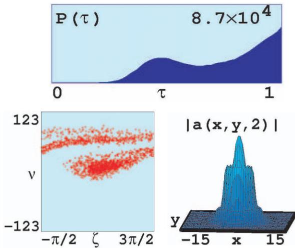
Figure 2: Simulation results for the SDL FEL with a -5% taper rate over the last 2.4 m of the undulator. On the top is the evolution of the optical power,  $P(\tau)$ . On the lower left is the final electron phase space as described in the text, with sample electrons shown in red. On the lower right is the final optical wavefront,  $|a(x, y)|$ , at the output mirror.
