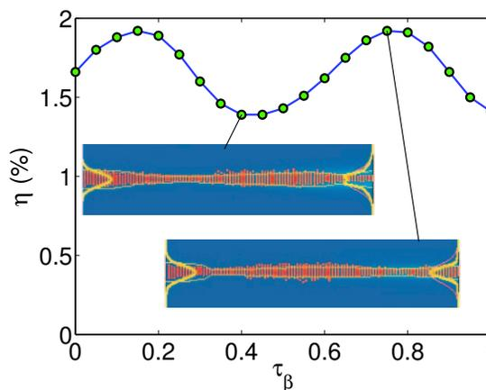
Figure 10: Extraction  $\eta$  vs. electron beam focus position  $\tau_\beta$  for the proposed LANL FEL. The inset plots show the evolution of the electron beam and the optical mode at  $\tau_\beta = 0.4$  (top) and  $\tau_\beta = 0.75$  (bottom).
