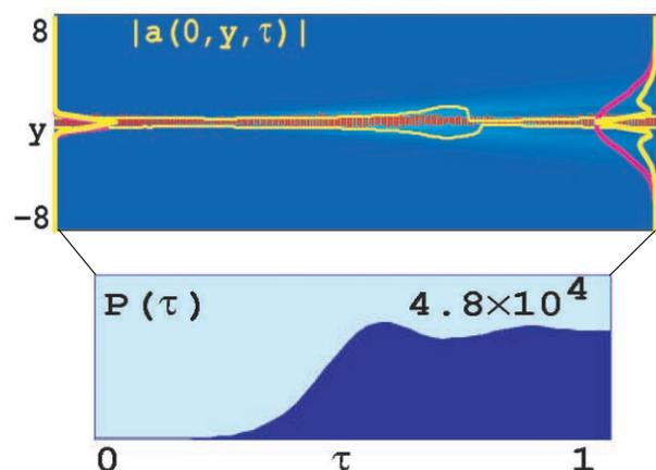
Figure 1: Simulation results for the SDL FEL with no taper. On the top is the evolution of the amplitude profile  $|a(y)|$ , as described in the text. On the bottom is the evolution of the dimensionless optical power  $P(\tau)$  from the beginning ( $\tau = 0$ ) to the end ( $\tau = 1$ ) of the undulator. The maximum value of the power is indicated in arbitrary units.
