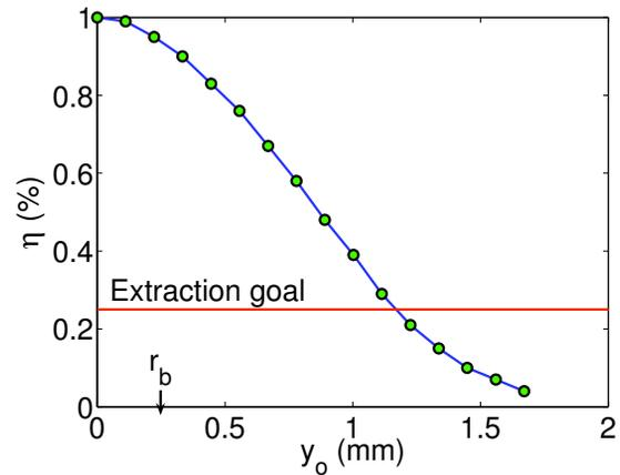
Figure 6: Extraction  $\eta$  vs. electron beam shift  $y_0$  for the proposed BNL FEL. The extraction goal is exceeded for all values of  $y_0 < 1.2$  mm, well beyond a typical experimental tolerance of  $\approx 50 \mu\text{m}$ , and much greater than the electron beam radius  $r_b = 0.25$  mm.
