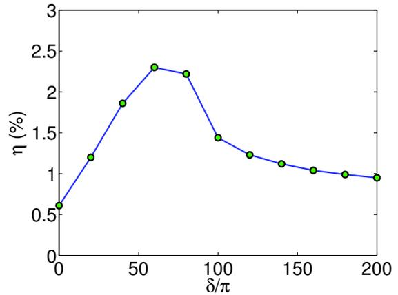
Figure 3: Extraction  $\eta$  versus phase acceleration  $\delta$  for the SDL FEL, with a linear taper over the last 5 m of the undulator. The maximum extraction  $\eta = 2.3\%$  is achieved for  $\delta = 60\pi$ , which corresponds to  $\Delta K/K \approx -7\%$ .
