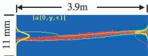
Figure 9: Optical field evolution for the proposed BNL FEL. Initial conditions are chosen so that the electron beam is tilted by  $\theta_y = 0.9$  mrad at the center of the undulator. The tilt appears exaggerated due to the different horizontal and vertical scales. Notice that the optical mode (narrow yellow contour line) follows the tilted electron beam (red).
