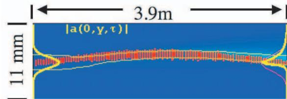
Figure 7: Optical field evolution for the proposed BNL FEL. Initial conditions are chosen so that the electron beam (shown in red) is shifted off-axis by  $y_0 = 1$  mm at the center of the undulator. Betatron focusing bends the beam back towards the axis at the ends of the undulator. The horizontal and vertical axis scales are quite different, as indicated. Notice how guiding enables the optical mode (narrow contour line) to follow the electron beam as it shifts off axis.
