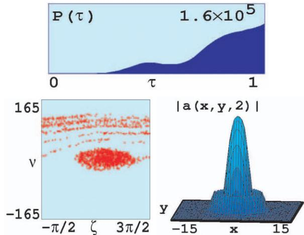
Figure 4: Simulation results for the SDL FEL, with a -7% taper rate over the last 5 m of the undulator.
