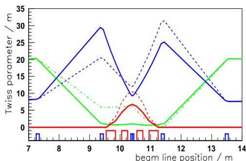
Figure 2: Horizontal (blue) and vertical (green) beta functions and dispersion (1000 times enhanced, red) of the deflecting chicane. The value of  $m_{56}$  is tuned to  $6.5 \cdot 10^{-5}$  (solid line) and  $26 \cdot 10^{-5}$  (dots), colours of magnets as described in fig. 1.
