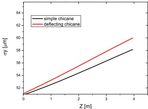
Figure 6: The development of the vertical electron beam size(rms) along the first radiator for both dispersive sections.
