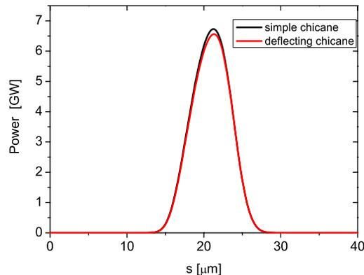
Figure 4: The radiator output power of the first stage of the medium-energy FEL for both dispersive sections. There exists a small difference between both cases, which is negligible concerning the seeding of the next section.
