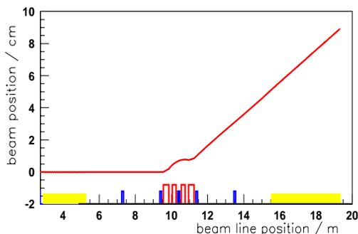
Figure 1: Horizontal trajectory of the electron beam as a function of beam line position. The red line shows the trajectory for the deflecting chicane (dipoles in red, quadrupoles in blue and undulators in yellow colours).
