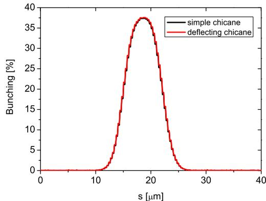
Figure 3: The bunching at the entrance of the first radiator of medium-energy FEL along the bunch for both dispersive sections. Both dispersive sections produces the optimal density modulation for the given energy modulation.
