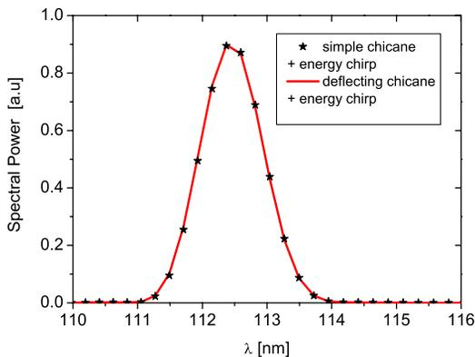
Figure 7: Spectrum of the output radiation for both dispersive sections. There is a shift in the wavelength due to the energy chirp. This is independent of the dispersive section.
