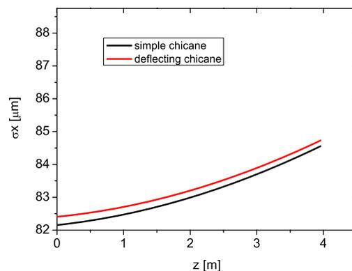
Figure 5: The development of the horizontal electron beam size (rms) along the first radiator for both dispersive sections. The difference between the beam sizes is less than 0.5 % and can be neglected.
