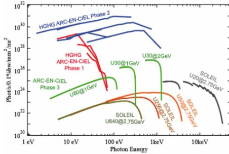
Figure 1 : Peak brilliance. Phase 1 : HHG radiation + seeding wavelength,  $P_{seed} = 100$  kW for HHG harmonics  $n^{\circ}7-9$ , 600 kW for  $n^{\circ}3-5$ . 1 kA,  $F = 0.1$ . Phase 2 : HHG radiation 1.5 kA,  $1.35 \pi$  mm.mrad, 0.0004% slice energy spread, 200 fs,  $\beta = 2$  m,  $F = 0.088$ . Phase 3 : spontaneous emission of undulators of period 30 and 80 mm calculated with SRW. Undulator period length in mm in ID name.
