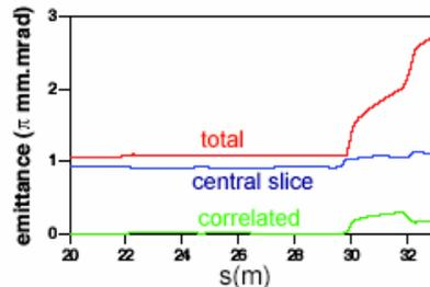
Figure 2 : Evolution of the emittance along the chicane. Chicane parameters: total length: 10 m,  $R56=0.15$  m, dipole length : 0.3 m. First dipole at  $s=23$  m.
