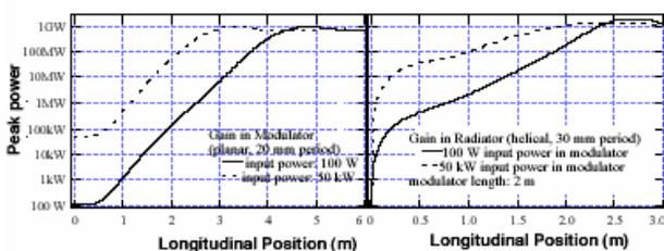
Figure 6: Steady-state GENESIS simulations for ArcEnCiel phase 1, 1 – 1 HHGG scheme, 266 nm seed: a) gain in modulator, b) gain in radiator (30 mm period helical mode).
