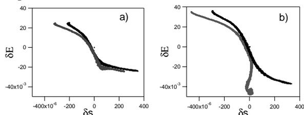
Figure 3 : Longitudinal phase space representation for a laser pulse length of a) 20ps, b) 40 ps for different voltages of the harmonic cavity. Black (resp. grey):  $E_H=22$  (resp. 20)MV/m.
