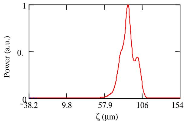
Fig. 7. Longitudinal profile of the radiation power at the end of the second undulator.
