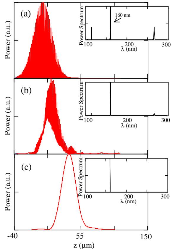
Figure 2 Power and spectrum of the radiation at different positions in the undulator for the SPARC FEL seeded at 160nm. Seed signal (a), after the first undulator section (b), at the end of the undulator (c). Beam energy 200 MeV,  $K=1.226$ , the other beam parameters as in Table 1.
