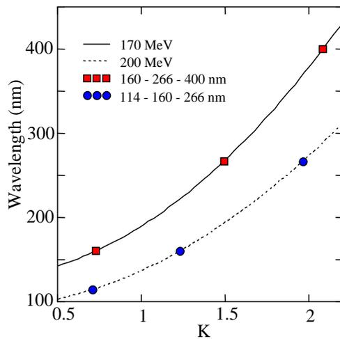
Figure 1: Seeded SPARC FEL operation wavelengths.
