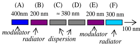
Figure 4 Fresh bunch injection technique layout.
