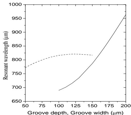
Figure 4: Plot of the free-space resonant wavelength  $\lambda$  with groove depth (solid line) as well as groove width (dashed line). For the solid line, we have kept groove width =  $62 \mu\text{m}$ . For the dashed line, groove depth =  $150 \mu\text{m}$ .
