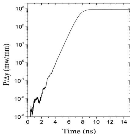
Figure 5: Plot of power per unit beam width in the surface mode as a function of time at the entrance of the grating for the optimized grating parameters.
