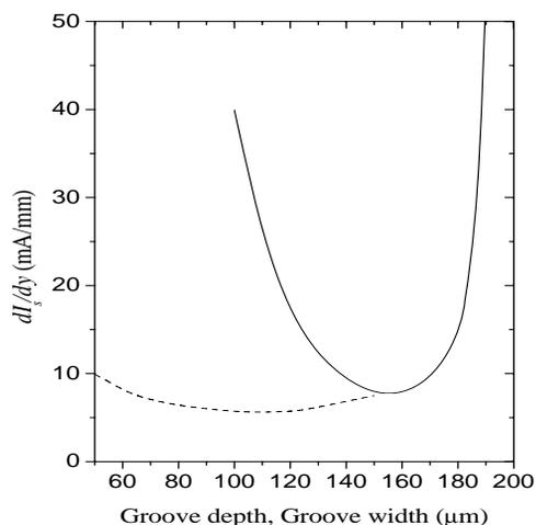
Figure 3: Plot of the start current density  $dI_s/dy$  with groove depth (solid line) as well as groove width (dashed line). For the solid line, we have kept groove width fixed at  $62 \mu\text{m}$ . For the dashed line, the groove depth is fixed at  $150 \mu\text{m}$ .
