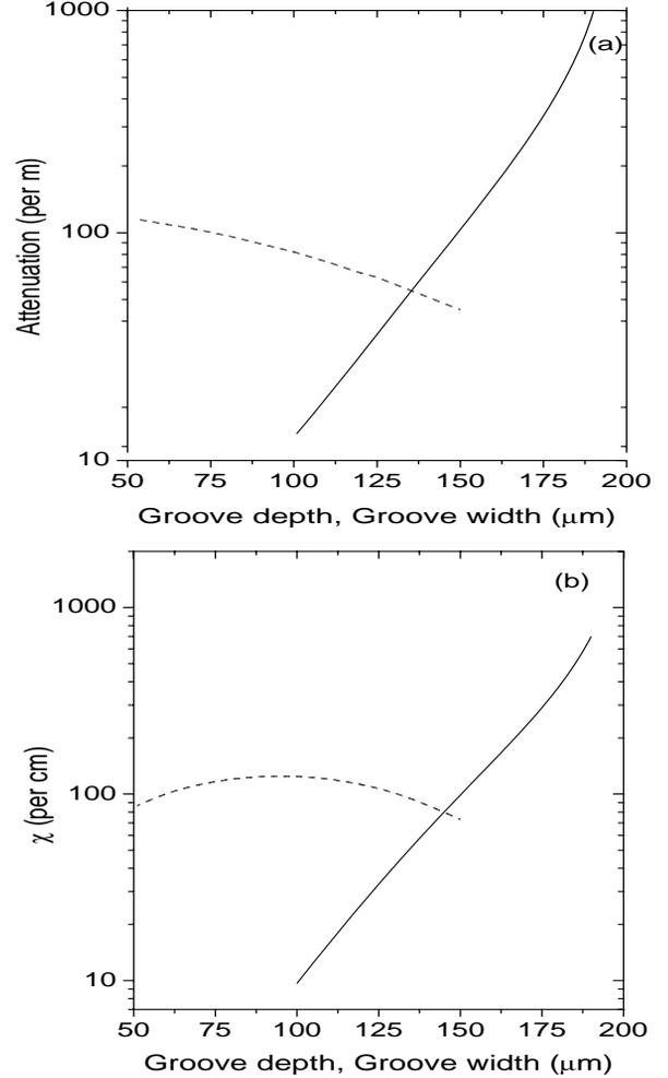
Figure 2: Plot of the real part of attenuation coefficient  $\alpha$  (a), and the  $\chi$  parameter (b) as a function of groove depth (solid curves) for groove width = 62  $\mu\text{m}$ , and as a function of groove width (dashed curves) for groove depth = 150  $\mu\text{m}$ .
