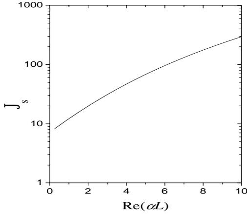
Figure 1: Plot of threshold dimensionless current  $\mathcal{J}_s$  as a function of the real part of the attenuation coefficient  $\alpha L$ .
