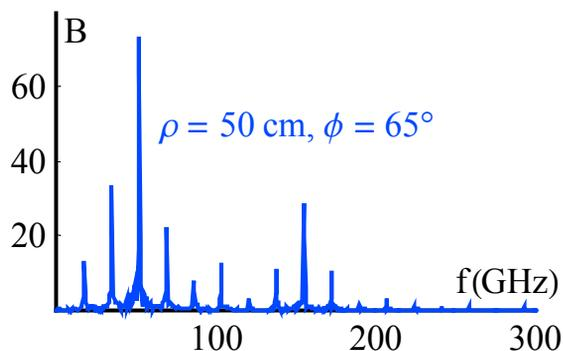
Figure 7. FFT of  $B_z$  following extrapolation. Third, sixth and ninth harmonics are more apparent.
