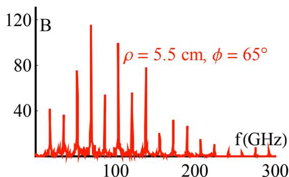
Figure 6. FFT of  $B_z$  at position indicated.
