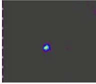
Figure 6: Transverse profile of the laser beam at the IP. Minimum beam waist found to be  $\sim 60 \mu\text{m}$ .
