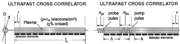
Figure 3: Ultra fast cross correlator. Pump-probe pulse coincidence is achieved via the difference in group velocities  $v_{\text{pu}}$  vs.  $v_{\text{pr}}$ . The pump modulates the Lorentz factor  $\gamma$  of the electrons. The Rayleigh waist diameters of the pump and probe pulses are both designated by  $d$ .
