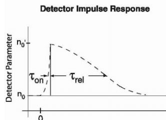
Figure 2: Temporal response of detector material to a pump impulse. The pump pulse modulates the physical parameter  $n_0$ .
