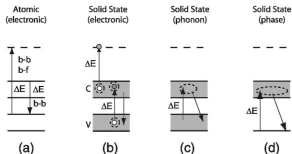
Figure 1: Various classes of excitation and relaxation processes in detector materials with activation energies  $\Delta E$  (a) Atomic transitions: b-b (bound-bound); b-f (bound-free), Relaxation processes include fluorescence, Auger, etc. (b) Solid state electronic transitions (conductor, semiconductor); V-valence; C-conduction. (c) Solid state phonon transitions. (d) Solid state phase transitions. Dashed ovals denote equilibration or relaxation processes
