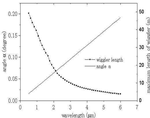
Figure 3: Angle  $\alpha$  and maximum wiggler length with respect to the radiation wavelength.
