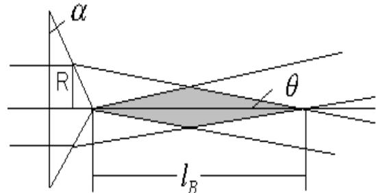
Figure 1: Bessel beam generation by axicon.
