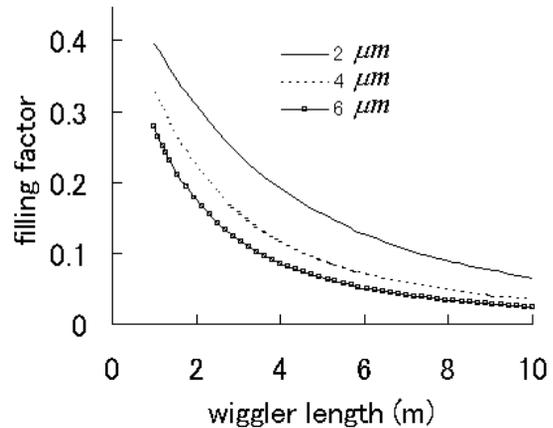
Figure 4: Filling factor with respect to the wiggler length for different wavelength.
