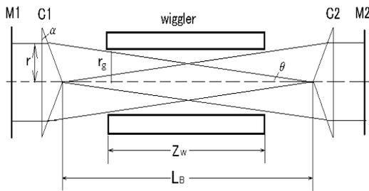
Figure 2: Conceptual design of a Bessel beam cavity for free-electron laser.
