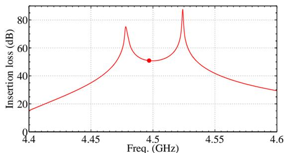
Figure 4: Insertion loss of the coaxial harmonic filter around the third harmonic frequency.
