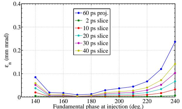
Figure 9: Normalized emittance vs. injection phase for optimum harmonic phase.
