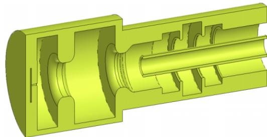
Figure 1: Cross-section view of the 1.5-GHz 1.5-cell RF cavity with the harmonic filter in the coaxial input feed.
