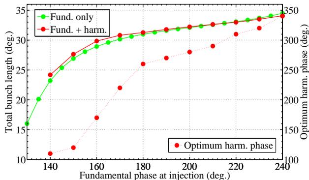
Figure 11: Total bunch length and optimum harmonic injection phase vs. fundamental injection phase.
