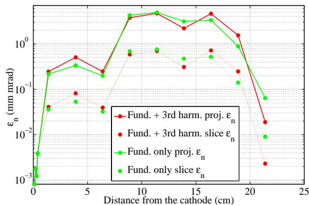
Figure 12: Normalized projected emittance and slice emittance (10-ps slice) vs. distance from cathode.
