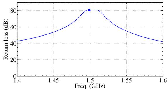
Figure 3: Return loss of the coaxial harmonic filter around the fundamental frequency.
