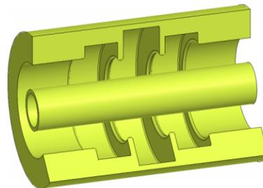
Figure 2: Cross-section view of the coaxial harmonic filter.
