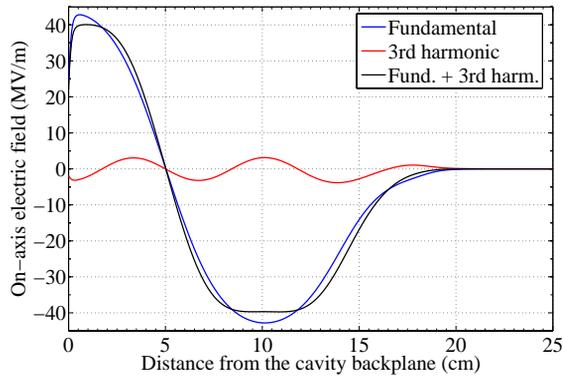
Figure 7: On-axis electric fields for the fundamental  $\pi$ -mode, the  $TM_{012-\pi}$  mode and their sum.
