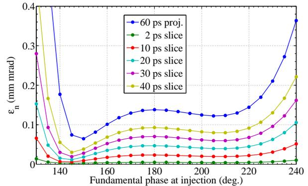
Figure 8: Normalized emittance vs. injection phase for the fundamental mode only.
