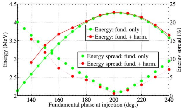
Figure 10: Average energy and energy spread vs. injection phase for fundamental alone and fundamental + harmonic.
