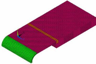
Figure 3: ANSYS FE simulation model for the vacuum chamber.
