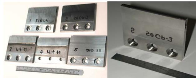
Figure 5: After machining (left 1: 316LN, 2: 20Cb-3, 3: Nitronic 33, 4: Nitronic 40, 5: 310S; right 20Cb-3)
