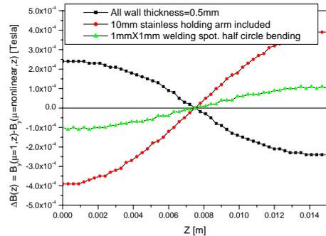
Figure 8: Absolute change of magnetic fields from the FE simulations in the half period along the beam direction.
