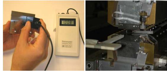
Figure 1: Test setups for measurement of magnetic permeability using a Ferromaster (left) and variation of applied magnetic fields using undulator A (right).
