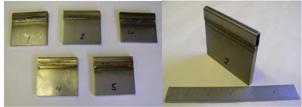
Figure 4: After welding (left 1: Nitronic 33, 2: 20Cb-3, 3: Nitronic 40, 4: 316LN, 5: 310S; right 20Cb-3)
