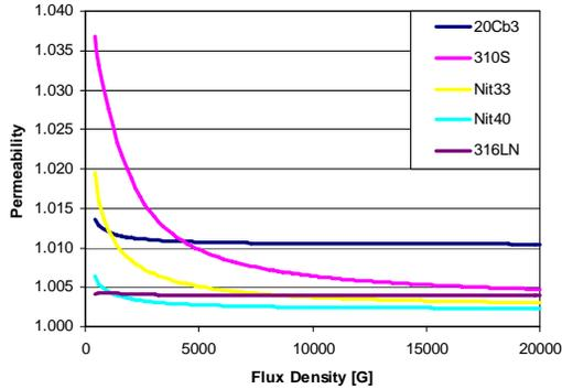
Figure 6: Magnetic permeability (without cold work) measured with Lakeshore’s 7400 series vibrating sample magnetometer.
