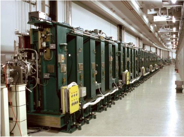
Figure 10: 25-m long IVU installed in the LSS in SPring-8.
