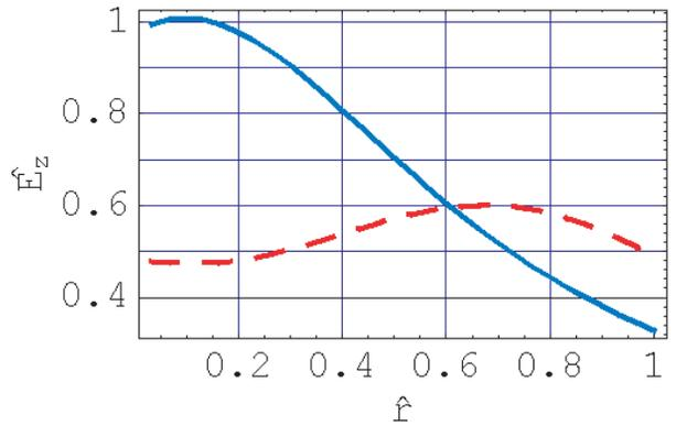
Figure 1: Example of Figs. 10 and 11 of Ref. [5]. The initial density modulation is  $\hat{a}_{1d} = e^{-\hat{r}^2/(2\sigma^2)}$  with  $\sigma = 0.1$ , and  $q = 1$ . The solid curve (blue) is at  $\hat{z} = 0$ , and the dashed curve (red) is at  $\hat{z} = 10$ . Notations have same meaning as in Ref. [5], the  $\hat{E}_z$  is normalized.
