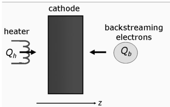
Figure 3: One dimensional heat conduction model.
