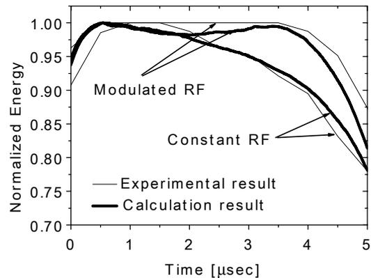
Figure 9: Experimental and calculation results of beam energy
