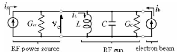
Figure 2: Equivalent circuit model.
