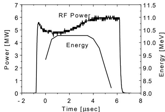
Figure 5: Beam energy and RF power fed into the gun (modulated RF).
