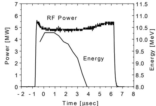
Figure 4: Beam energy and RF power fed into the gun (constant RF).
