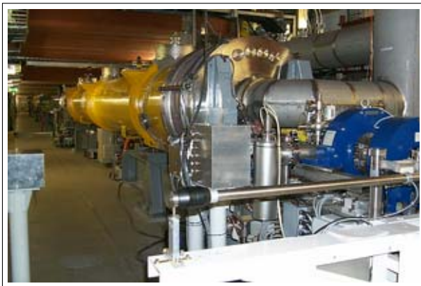
Figure 2: View of the VUV-FEL injector from the RF gun down the accelerator. The RF gun is inside the blue solenoids in the foreground. The yellow cryostat is the TESLA module used as a booster.
