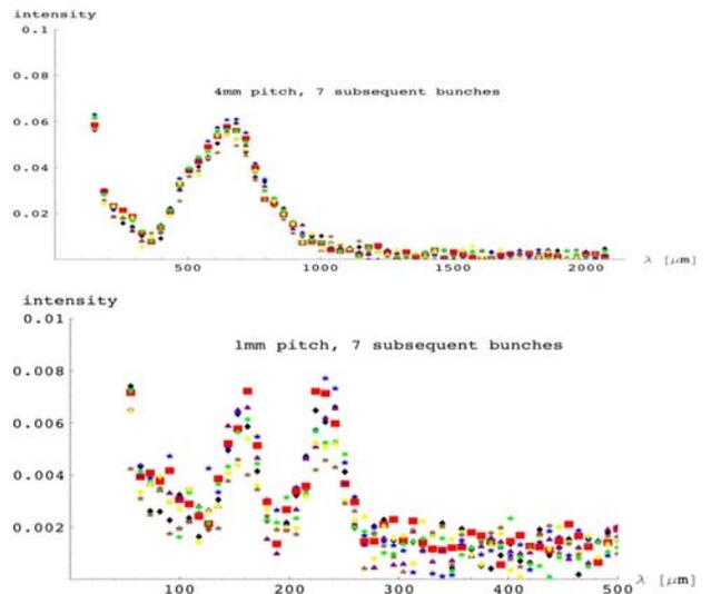
Figure 5. Bunch to bunch spectra made by TG spectrometer.
