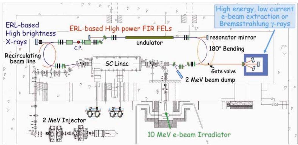
Figure 1: Layout of Multi-purpose Quantum beam generation system.
