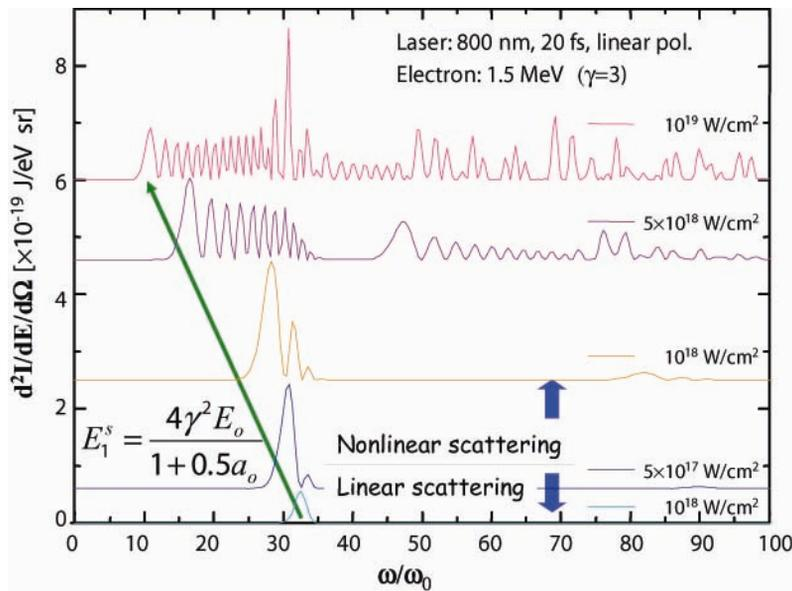
Figure 6: The angular spectra of Compton backscattered X-rays at  $\phi=0$  for different laser intensities
