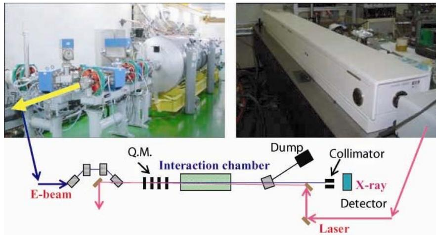
Figure 2: Layout for 1keV Compton X-ray generation.
