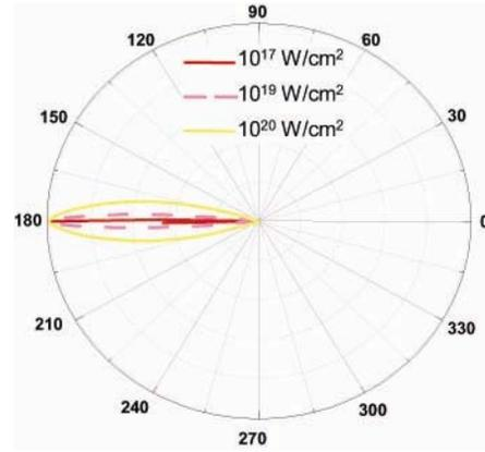
Figure 5: The angular distribution of Compton backscattered X-rays for different laser intensities.
