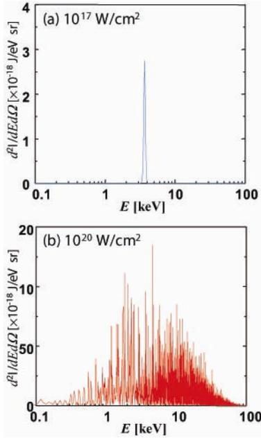
Figure 4: Compton scattered radiation at  $\phi=0$ . (a) linear scattering and (b) non-linear Compton.
