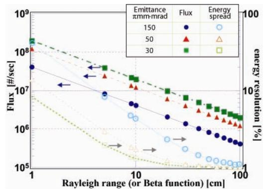
Figure 3: The expected Compton X-rays depending on the emittance and the beta function of electron beam.
