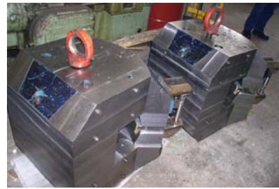
Figure 3: NESTOR bending magnet after reconstruction.
