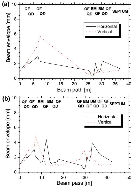
Figure 1: Calculated beam envelopes in the electron-beam transport systems before (a) and after (b) the improvement. The beam sizes, angular spread and energy spread at the last beam position monitor in the Linac room are assumed to be 1 mm, 1 mrad and 0.5%, respectively.
