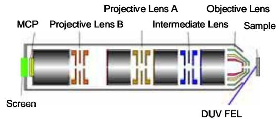
Figure 6: Schematic layout of the PEEM system.
