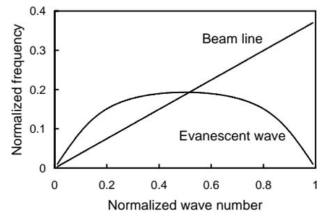
Figure 1: Dispersion relation and beam line for a typical grating.
