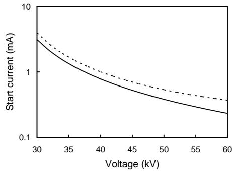
Figure 4: Predicted start current in the SP-FEL experiments at Dartmouth [8] including losses (solid curve) and ignoring losses (dotted curve).
