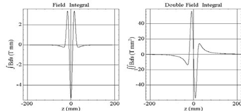
Figure 8: First and second field integrals along axis.
