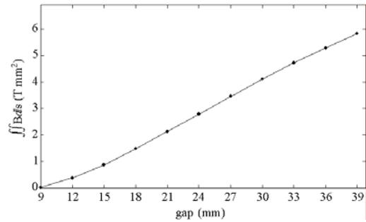
Figure 14: Second field integral as a function of the gap.
