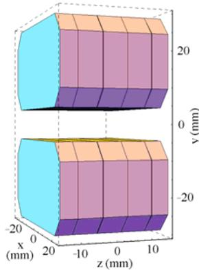
Figure 11: Second configuration for the phase shifter (five horizontally cut magnets); the total length is 31 mm.
