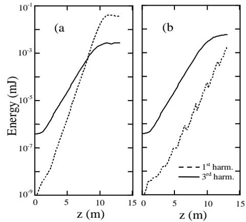
Figure 4: Pulse energy vs. longitudinal coordinate along the undulator. In (a) phase does not change along the undulator. In (b) phase shifts  $\phi = \pm 2\pi/3$  every 30 periods, with alternated sign, are introduced.
