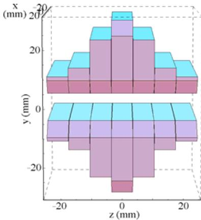
Figure 6: First configuration for the phase shifter (seven horizontally cut magnets); the total length is 49 mm.
