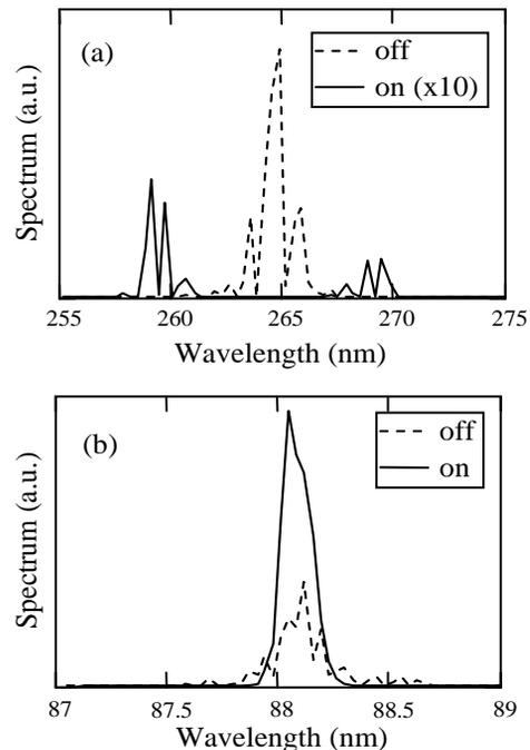
Figure 5: First (a) and third (b) harmonic spectrum at the end of the undulator with (continuous line) and without (dashed line) phase shifts. In (a) the first harmonic spectrum suppressed by the shifts has been multiplied by a factor 10.
