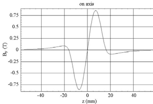
Figure 12: Vertical component of the magnetic field.
