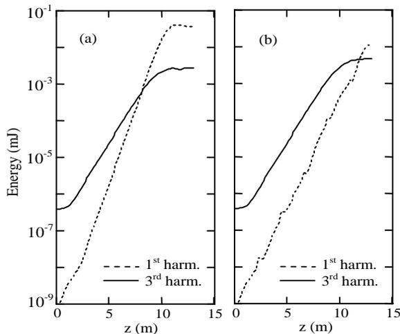
Figure 3: Pulse energy along the SPARC undulator in seeded mode at the third harmonic ( $\lambda = 88$  nm, corresponding to a FEL resonance at 264 nm). In (a) phase does not change at each gap. In (b) phase shifts  $\phi = \pm 2\pi/3$ , with alternated sign, are introduced at each gap.
