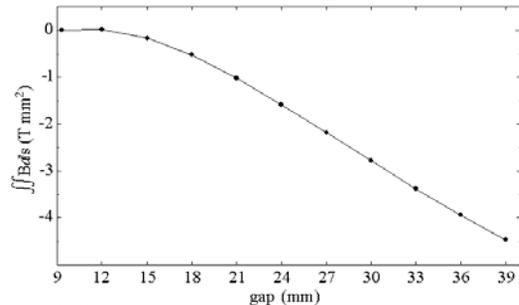
Figure 9: Second field integral as a function of the gap.
