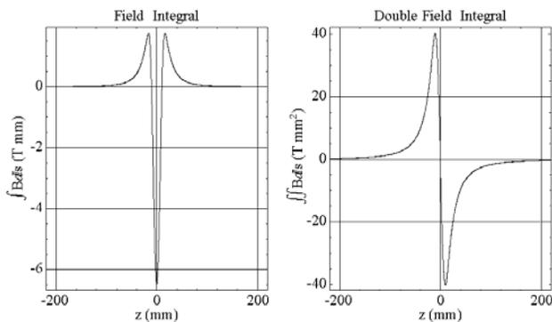
Figure 13: First and second field integrals along axis.
