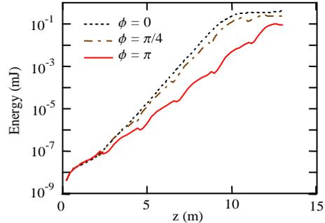
Figure 1: Energy along the SPARC undulator for different phase shifts  $\phi$  at the gaps, in SASE mode ( $\lambda = 500$  nm).
