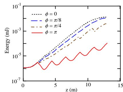
Figure 2: Energy along the SPARC undulator for different phase shifts  $\phi$  at the gaps, in seeded mode ( $\lambda = 160$  nm, 15 kW input power, 100 fs pulse duration).
