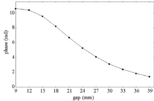
Figure 15: Phase correction as a function of the gap.
