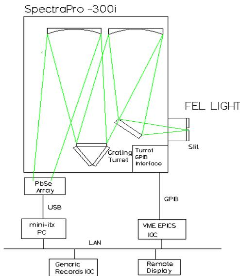
Figure 1: Spectrograph Hardware.
