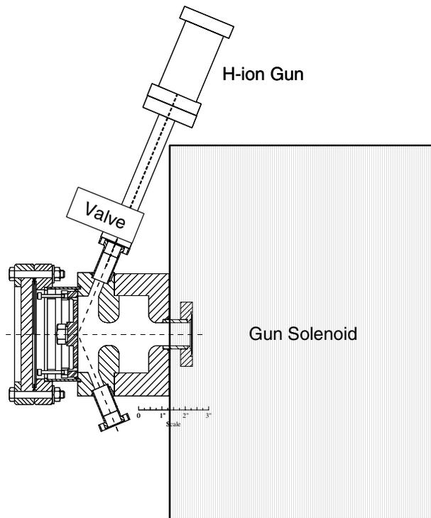
Figure 7: The proposed configuration for in-situ cleaning of the cathode in an s-band RF gun.
