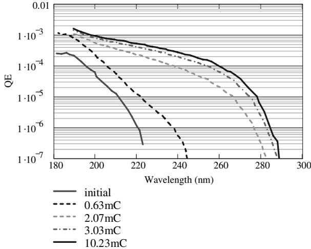
Figure 1: The QE for a copper sample vs. wavelength with increasing exposure to the H-ion beam.
