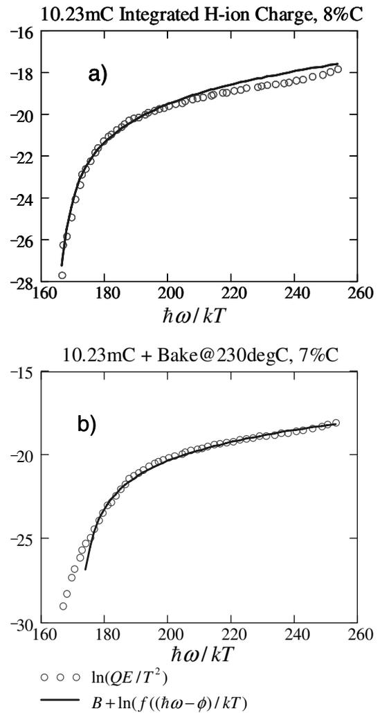
Figure 4: a) Fowler plot after final integrated exposure of 10.23mCoul. b) The result of heating the sample to 230degC.
