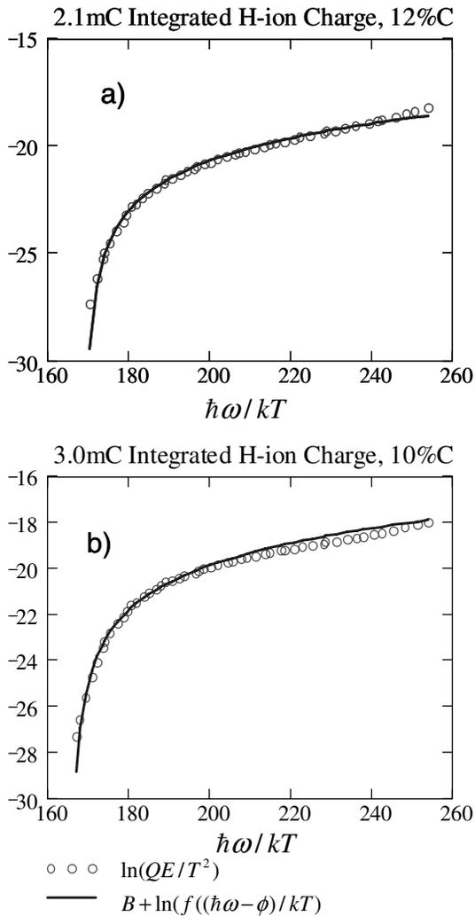
Figure 3: Fowler plots for sample exposed to a) 2.1mCoul of H-ions and b) after 3.0mCoul of H-ions.
