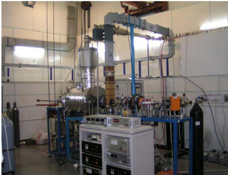
Figure 3: Layout of DC-SC photoinjector beam line
