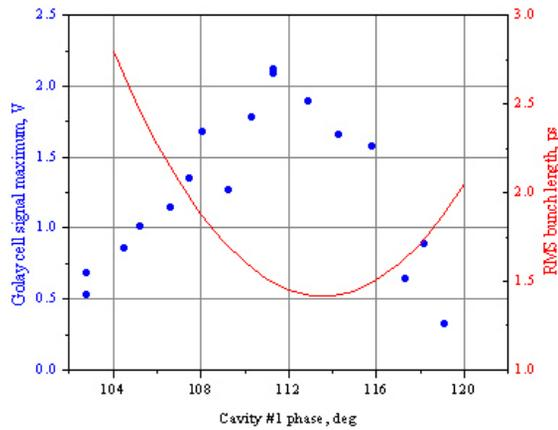
Figure 5: Measured Golay signals (dots) and RMS bunch length (line) as a function of the cavity #1 phase. The RMS bunch length is measured with the Martin-Puplett interferometer. The plot shows that the Golay cell signal alone is a useful tool to adjust different bunch length conditions of the electron beam.
