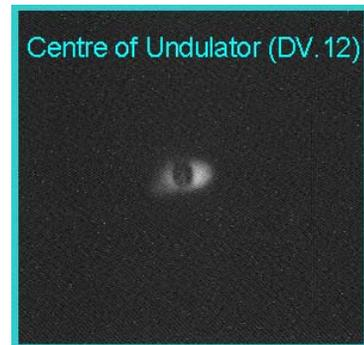
Figure 3: OTR view screen picture from the undulator. The picture shows the position and shape of the electron beam in the undulator. The diameter of the hole in the view screens is 1mm.
