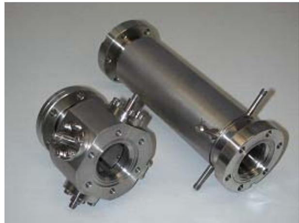
Figure 4: Picture of the  $1/4 \lambda$  and  $3/4 \lambda$  beam position monitors used at ELBE.
