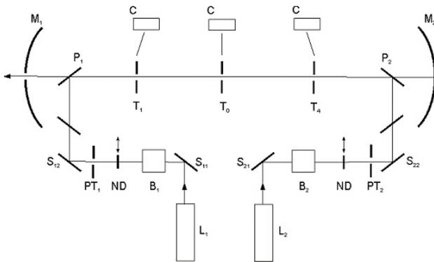
Figure 2: Schematic diagram of the optical cavity and components for the alignment system ( $M_j$ : cavity mirrors,  $P_i$ : pop-in mirrors,  $T_i$ : adjustment apertures,  $C$ : monitoring cameras,  $S_{ij}$ : steering mirrors,  $PT_i$ : iris diaphragm,  $ND$ : neutral density filters,  $B_j$ : beam expanders,  $L_j$ : He-Ne alignment lasers)
