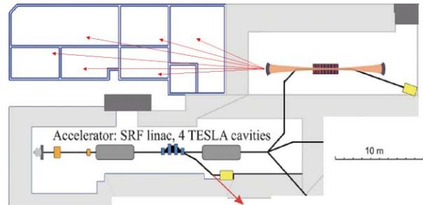
Figure 1: Schema of the ELBE main accelerator hall, the FEL cave and the user labs. Each of the two acceleration modules contains two nine cell Tesla cavities. The electron energy for operating the FEL between 22  $\mu\text{m}$  and 4  $\mu\text{m}$  ranges from 15 MeV to 34 MeV. The permanent magnet undulator U27 (27 mm period) consists of two segments and has a minimum gap of 13.8 mm. The infrared laser beam can be distributed to different laboratories.
