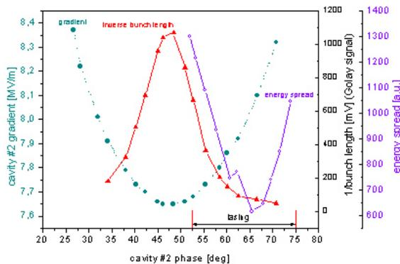
Figure 6: Plot of the energy spread and Golay signal measured as function of cavity #2 phase for the ELBE setup with one accelerating module.
