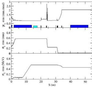
Figure 3: Horizontal emittance, pulse duration and energy spread of the electron bunch for an initial charge of 1 nC. Case of a laser pulse of 20 ps, a bunch compression of 300 fs.
