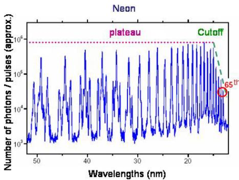
Figure 5: Typical harmonics spectrum produced in a Neon jet. In the plateau region, the harmonics intensities are almost constant with harmonic order. For higher orders, the intensities decrease rapidly in the "cut-off" zone.
