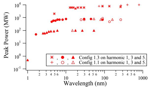
Figure 8: HGHG radiation for ARC-EN-CIEL Phase 2. 1.5 kA, 1.35  $\pi$  mm.mrad, 0.0004% slice energy spread, 200 fs, beta=2 m, filling factor = 0.088.
