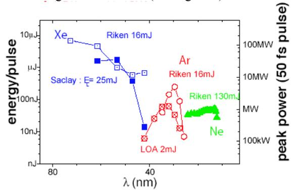
Figure 6: Performances of the harmonics produced in gases.
