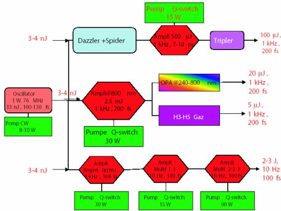
Figure 4: The laser system for ARC\_EN-CIEL phase 1.
