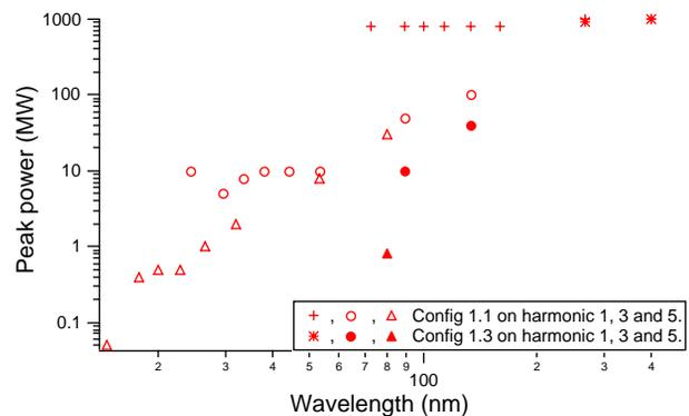
Figure 7: HGHG radiation + for the seeding wavelength, • for the third harmonic, Δ for the fifth harmonic. 1 kA peak power. Filling factor = 0.1
