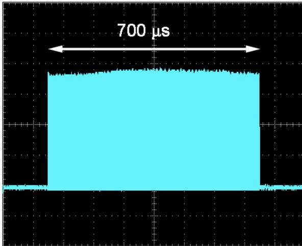
Figure 4: Output pulse trains of the OPCPA system containing 700 micropulses
