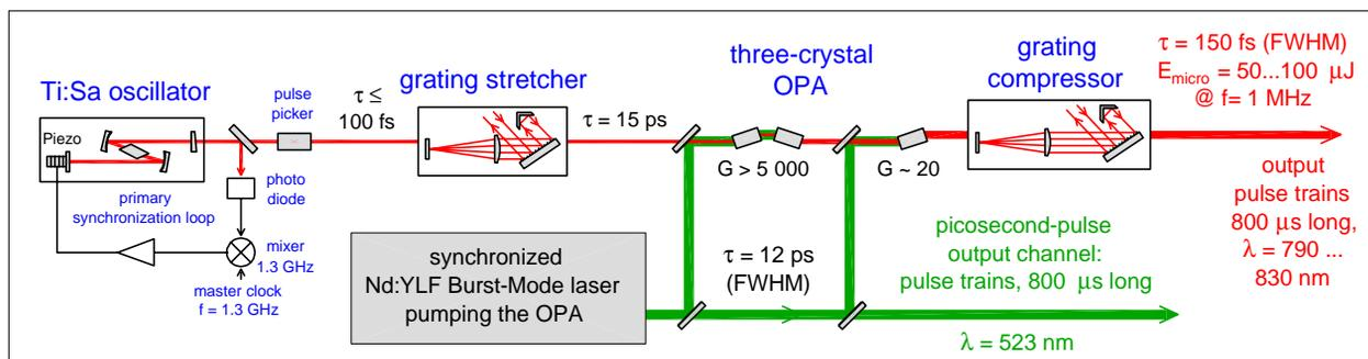
Figure 1: Basic scheme of the OPCPA laser system
