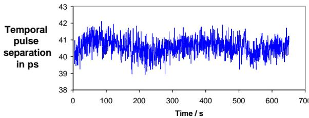
Figure 6: Synchronization jitter between OPCPA and light from a bending magnet measured with a streak camera
