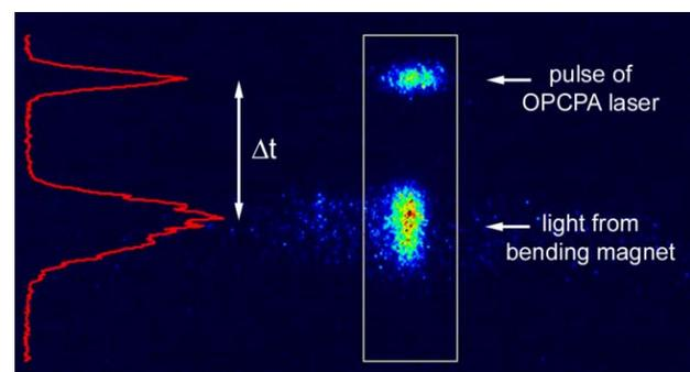
Figure 5: Streak camera image obtained by simultaneously imaging the pulses from the OPCPA system and the light from a bending magnet onto the photocathode of the synchroscan streak camera. (The time axis goes in vertical direction)
