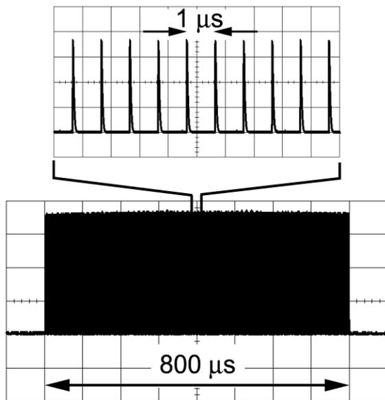
Figure 2: Pulse trains from a Nd:YLF burst-mode laser which is used as the pump laser of the optical-parametric amplifier
