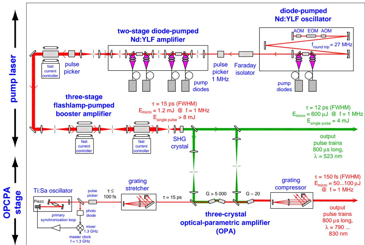
Figure 3: Optical layout of the OPCPA laser system
