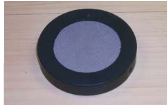
Bolometric Detector with Filter Wheel
