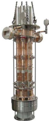
Figure 3: Prototype MBK for TESLA
