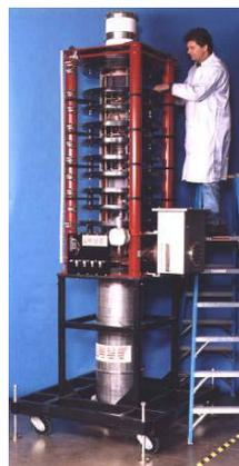
Figure 1: VKP-7958A Klystron for DESY
