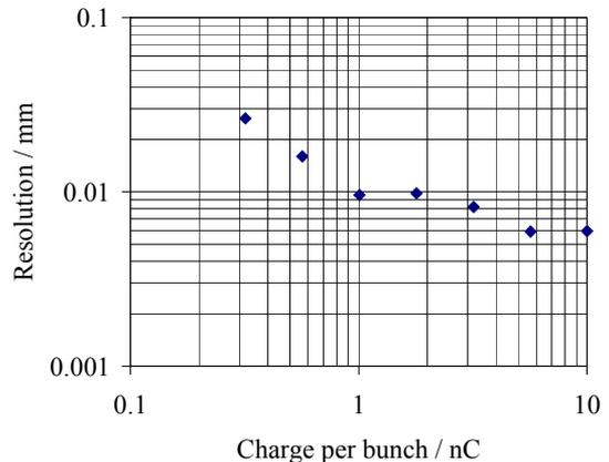
Figure 4: Laboratory measurement of pulsed to pulse position fluctuation for a typical stripline pickup with position sensitivity of  $0.1 \text{ mm}^{-1}$ .
