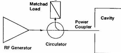
Figure 1: RF system of the standing wave accelerator[1].
