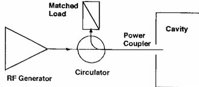
Figure 1: RF system of the standing wave accelerator[1].
