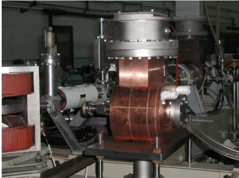
Figure 9: Picture of the new RF-gun.
