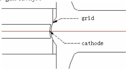
Figure 4: Structure of the RF-gun near the cathode.
