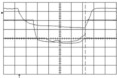
Figure 3: Electron beam waveform of thermionic RF-gun(<ch1>).
