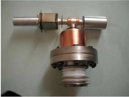
Figure 8: Picture of control grid electron gun.
