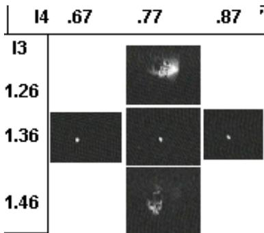
Figure 3: Spot at S2 for various currents  $I_3$  and  $I_4$ , for  $I_1=1.26$  A and  $I_2=1.14$  A.
