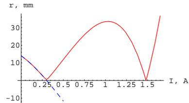
Figure 2: Radius  $r_2$  of beam at S2 vs. current  $I = I_1 = \dots = I_4$ ; beam has waist at S1, with emittance  $\varepsilon = 6$  mm mrad, and radius  $r_1 = 14$  mm. Blue dashed line is approximation for  $r_2$  in Eq. (21). Note that, at minima, the radius of beam is very small, yet non-zero.
