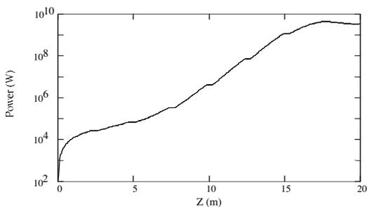
Figure 5: Power vs.  $z$  for the 10 nm SPARXINO SASE-FEL source, GENESIS simulation (slice energy spread  $8 \cdot 10^{-4}$ , slice norm. emittance 1 mm mrad, slice peak current 2 kA, undulator parameter  $K=2.2$ )
