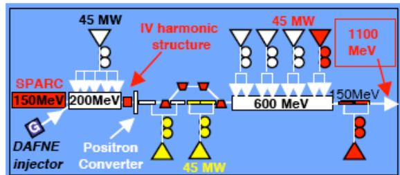
Figure 6: Scheme of the Frascati linac upgrade for SPARXINO and DAΦNE operation. Existing elements (white). Additional SPARXINO elements (red). Additional elements for positron acceleration (yellow).
