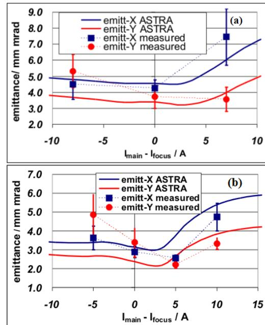
Figure 1: Projected normalized emittance as a function of the main solenoid current  $I_{\text{main}}$ : (a) for a bunch charge of 0.5 nC and a gaussian laser pulse with a length of 6.3 ps FWHM, and (b) for a bunch charge of 1.0 nC and a flat top laser pulse with a length of 23 ps FWHM.  $I_{\text{focus}}$  denotes the solenoid current to focus the beam on the position of the slit mask.
