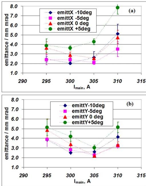
Figure 2: Projected normalized horizontal (a) and vertical (b) emittance for different main solenoid currents and gun phases  $\phi - \phi_m = -10^\circ, -5^\circ, 0^\circ, +5^\circ$ . The bunch charge is 1.0 nC.
