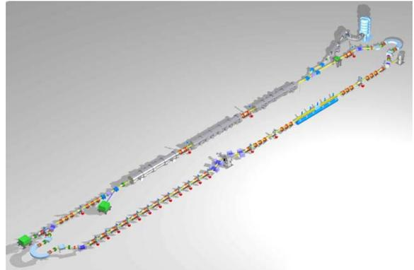
Figure 1. Layout of the IR Upgrade FEL in its final configuration. The beam starts at the injector at the upper right, is merged with the full energy beam in an injection chicane, accelerated up to as much as 160 MeV in three cryomodules, transported to the optical klystron, and from there back to the linac. At the exit of the linac the energy-recovered beam is separated from the accelerated beam and is dumped in a water-cooled copper dump.
