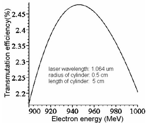
Fig. 3 Transmutation efficiency vs. electron beam energy
