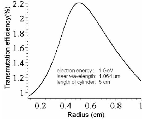
Fig. 2 Transmutation efficiency vs. radius of target
