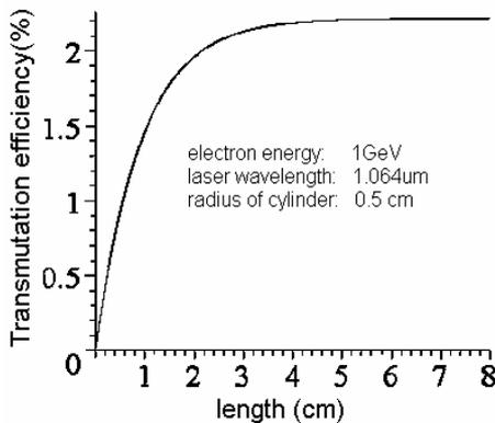
Fig. 1 Transmutation efficiency vs. the length of target
