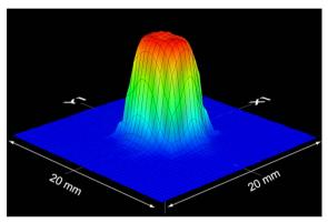
Fig. 8 : Current density profile of the 500 keV, 1.0 A beam.
