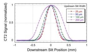
Fig. 6 : Beamlet profiles for different upstream slit width.
