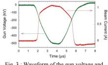
Fig. 3 : Waveform of the gun voltage and beam current.
