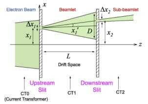
Fig. 5 : Principle of emittance measurement.
