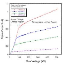
Fig. 4 : Current-voltage characteristic of the CeB<sub>6</sub> gun.
